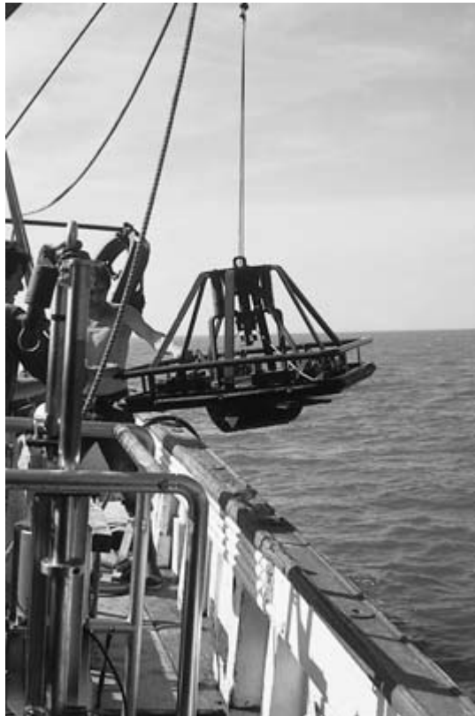
Fig. 8.1. Reineck box sampler. (A) The rectangular coring tube is closed by a knife edge actuated by pulling on the lever on the left. An attachment can be fitted to show the inclination and compass orientation of the core. Redrawn from Holme & McIntyre (1984). (B) The corer being lifted back on board. Photo courtesy of John Costello, Aquafact International Services Ltd., Galway, Ireland.
