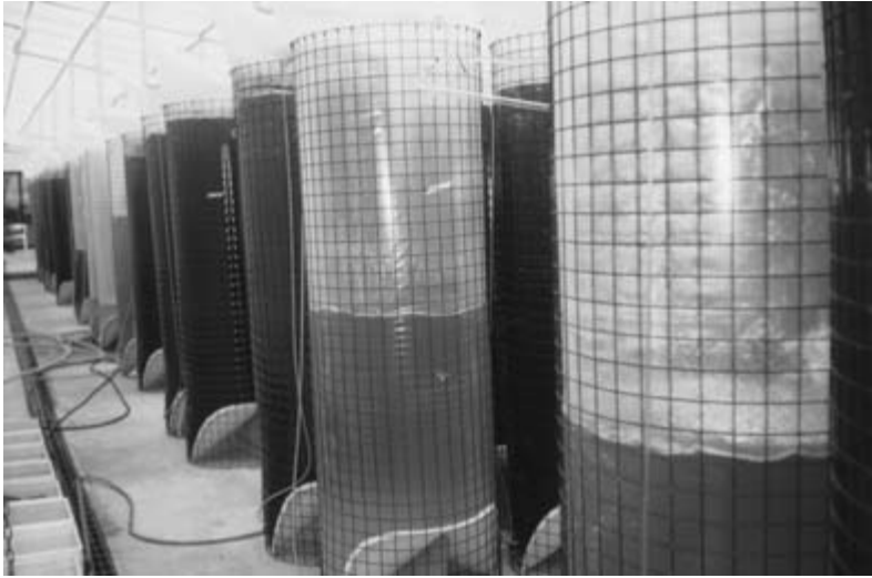
Fig. 9.2. Large, transparent plastic tubes used in the culture of microalgae. Photo courtesy of Kevin O Kelly, Lissadell Shellfish Co. Ltd., Sligo, Ireland.
