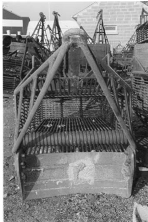
Fig. 8.4. (A) Scallop dredge with spring teeth and mounted six to a tow. From Hardy (1991). (B) Breton clam dredge (2 m long, 50 cm wide) used in NW France. This box-like dredge is made of long metal rods, and a sharp blade, shearing downwards, can be clearly seen at the lower part of the opening. Boats (10–15 m long) tow one dredge each side. Photo courtesy of M. Wilkins, Channel Marine Ltd., London.
